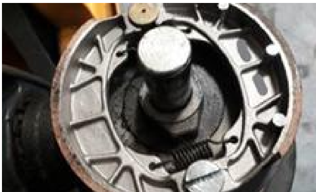
Uncovered asbestos containing brake assembly of an affected manual hand pallet truck imported from China.
